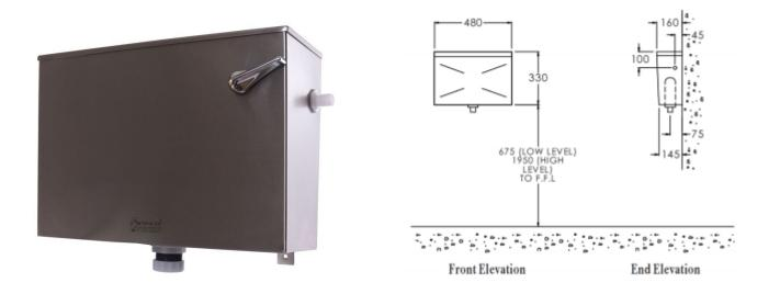
Model WC132 is a manual stainless steel cistern designed for use with our WC pans, with exposed surface mounting. This is suitable for low level installations with an internal overflow. These cisterns are manufactured from grade 304 stainless steel with all exposed surfaces polished to a satin finish. The cistern is supplied with a lid, flushing mechanism and a stainless steel 90 degrees flush pipe.
